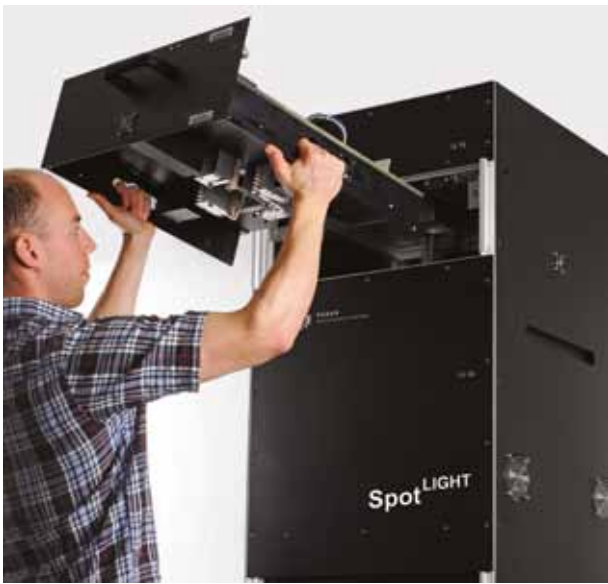
Figure 6. Tray drawer for lamp replacement in the Pasan Spot LIGHT series [2].
