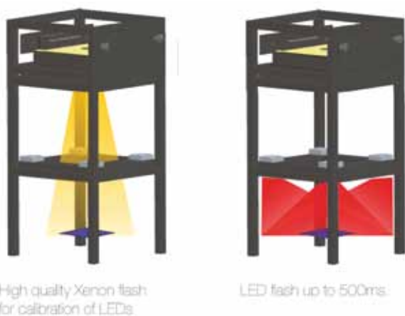
Figure 7. Measuring methodology of the new Pasan Spot LIGHT HighCap [2].
