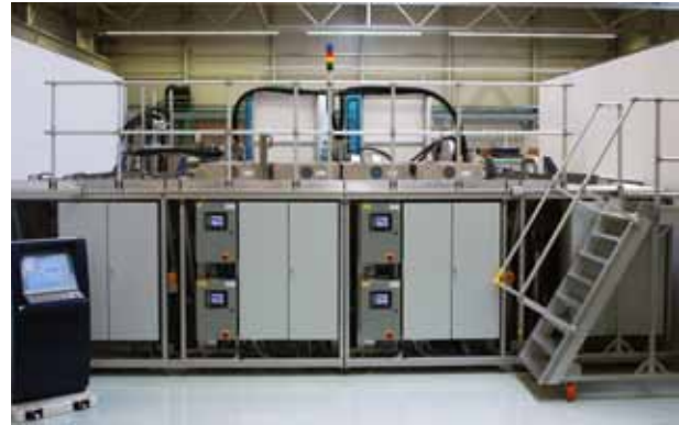
Figure 3. The Roth & Rau HELiA PVD tool is made up of two sputtering chambers – one for the TCO, with targets on the front and back sides, and the other for the metal, with targets only on the back side. The targets are mounted on rotating magnetrons [1].
