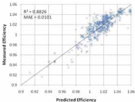
Figure 4. Correlation of the predicted efficiency and the measured efficiency [3].
