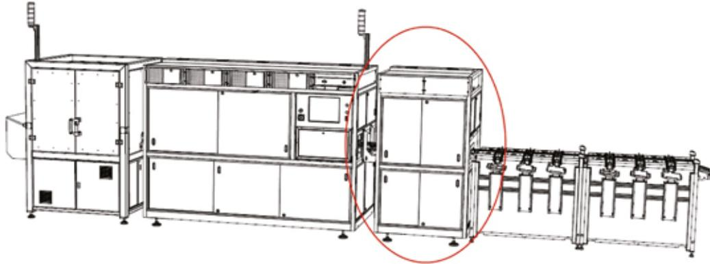
Figure 6. Hennecke Systems PL imaging module integrated in a Hennecke Systems wafer inspection system.
