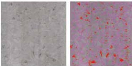
Figure 7. Automatic evaluation of crystal boundaries and dislocations (in the right-hand image, purple = grain boundaries with low lifetimes, and red = dislocation clusters).
