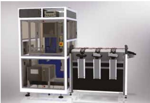
Figure 13. Manual loading and automatic sorting PL image inspection (Hennecke Systems GmbH).
