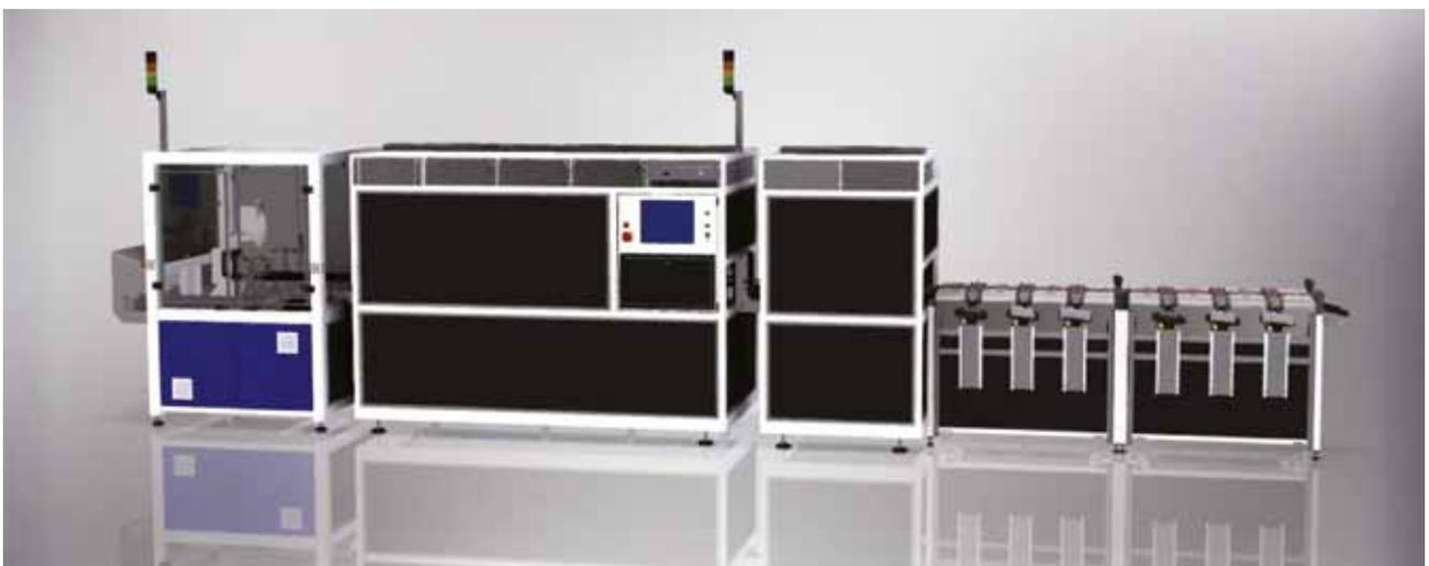
Figure 15. PL imaging module integrated with the He-WI-04 inspection system (Hennecke Systems GmbH).
