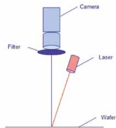
Figure 5. PL imaging system principle.
