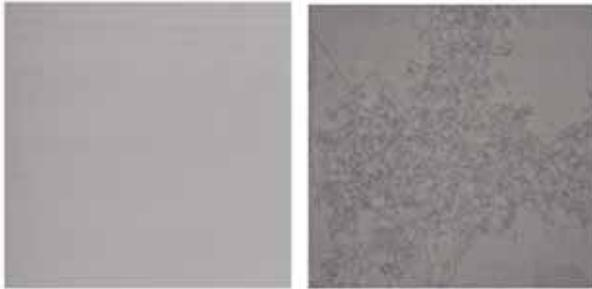
Figure 9. An obviously well-grown mono-cast wafer without any visually apparent crystal borders (left) may still contain lots of dislocations, visible in the PL image (right).
