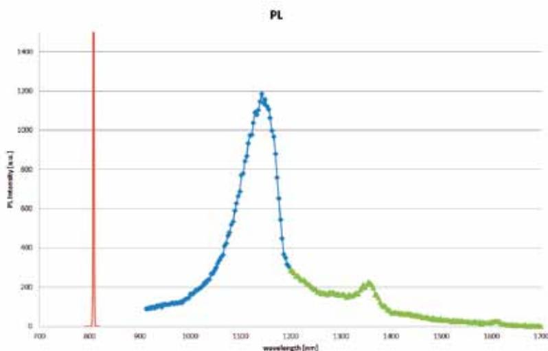
Figure 2. Spectrum of PL radiation: red = illuminating laser wavelength, blue = normal PL from band-band recombination, and green = PL light from band-defect recombination.
