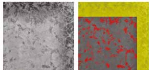
Figure 11. Automatic evaluation of the fraction of impurities, shown here at the corner of the wafer as dark regions along the top and right sides (in the right-hand image, yellow = impurity region, and red = dislocation clusters).
