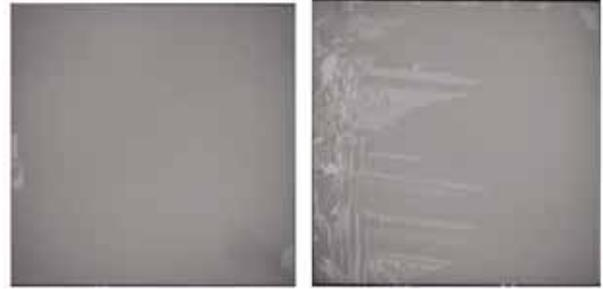
Figure 10. Visual images of a cast-mono wafer with high mono-fraction (left) and low mono-fraction (right).
