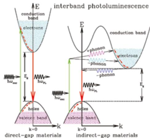
Figure 1. Band structure of direct and indirect band gap materials.
