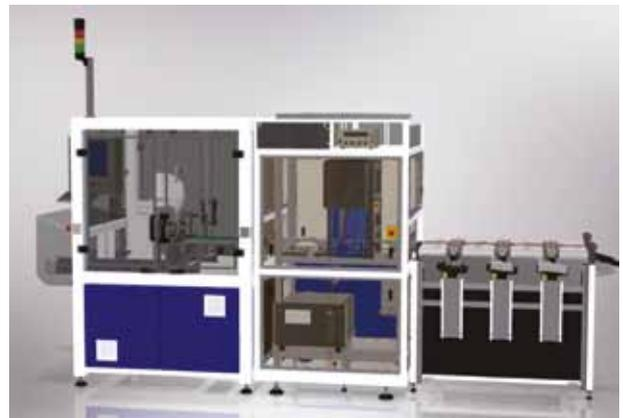
Figure 14. PL imaging module with stack loading and automatic sorting (Hennecke Systems GmbH).
