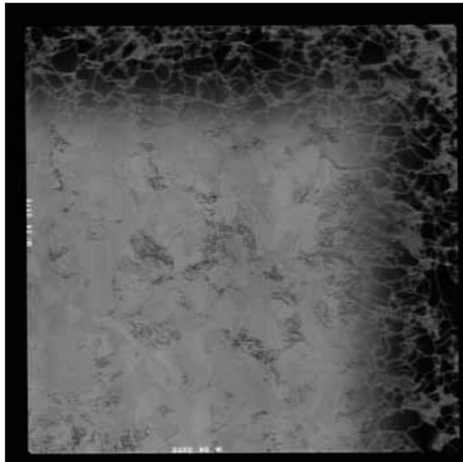
Figure 3. Impurities in this corner brick result in the dark areas seen here in the upper and right sides of the wafer. Dislocations result in dark lines.
