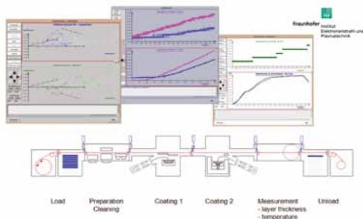
Figure 6. Process and control loop visualization.
