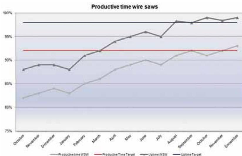
Figure 10. Improvement of productive time for Meyer Burger wire saws with automation.
