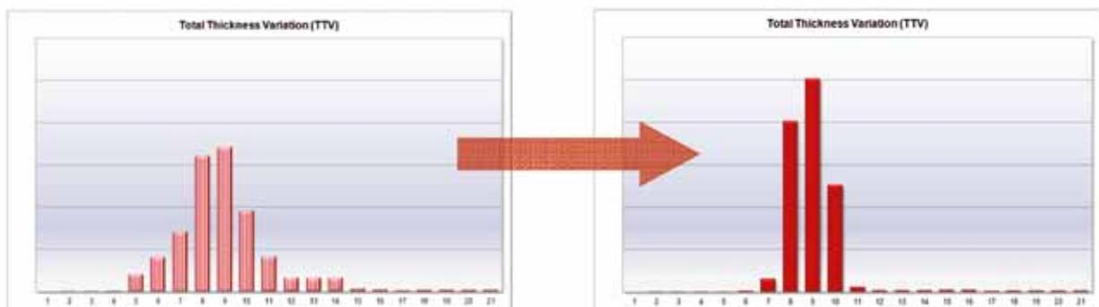
Figure 9. Comparison of TTV before and after deployment of automation.
