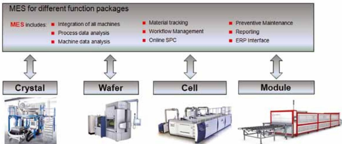
Figure 1. Integrated automation system for PV manufacturing.
