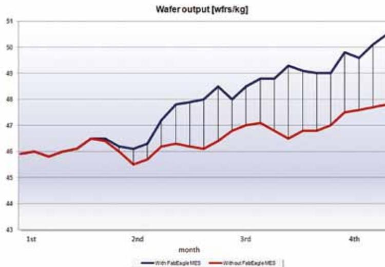
Figure 8. Increase in wafer output when APC is used in cropping.
