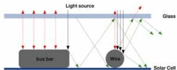
Figure 6. Reduced front wire shading and effective shading profile reduced to 64% [1].
