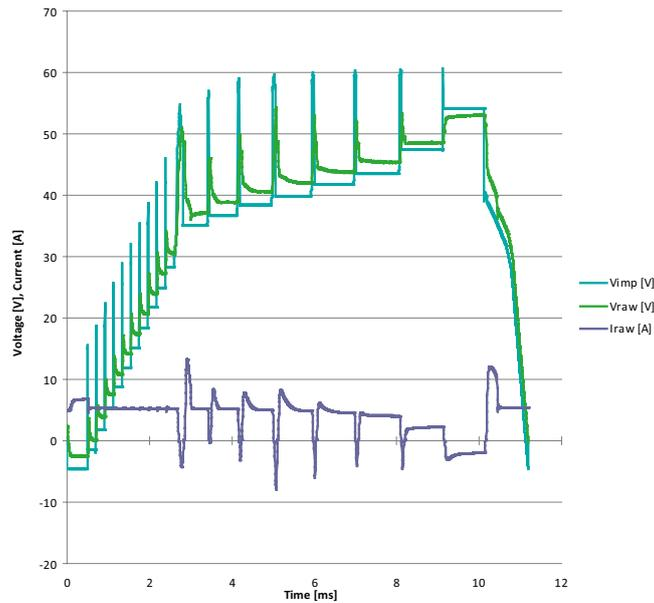
Figure 15. DragonBack applied voltage (blue), and the resulting measured voltage (green) and current (violet) for a commercial HJT module (type 1).
