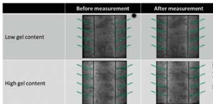
Figure 10. Electroluminescence images of a cell before and after measurement using the X Link method [7].
