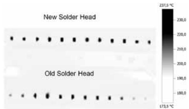
Figure 3. A thermal image, shown as a greyscale picture, for the new and old soldering heads. The temperature distribution has been almost completely equalized, especially in the border areas. This allows shorter soldering times as well as lower thermal stress to the cell.
