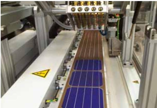
Figure 2. A Somont solder unit for two, three and five busbars.
