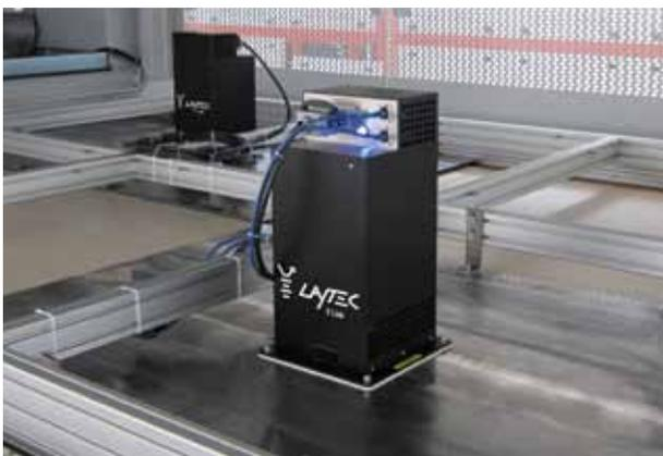
Figure 12. Integration of the X Link sensing head into the cooling press of a 3S Modultec laminator [8].
