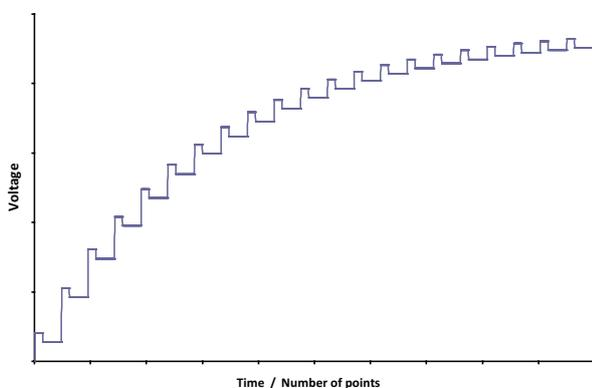
Figure 14. Typical DragonBack voltage ramp, including steps and overshoots.
