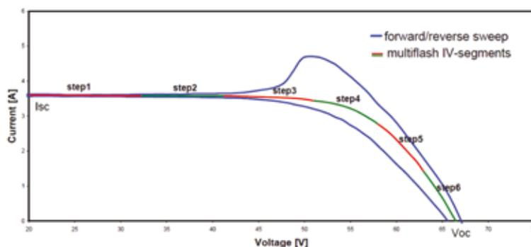
Figure 13. Forward and reverse I-V curves measured on a HiCap module with a linear sweep in a single 10ms flash (blue) compared to an MF measurement taken on the same module.
