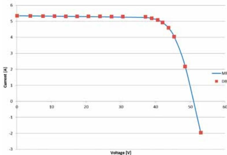
Figure 16. Comparison of the  $I$ - $V$  curves obtained with the DragonBack method (red squares) and the reference MF measurement (blue line) for a commercial HJT module (type 1).
