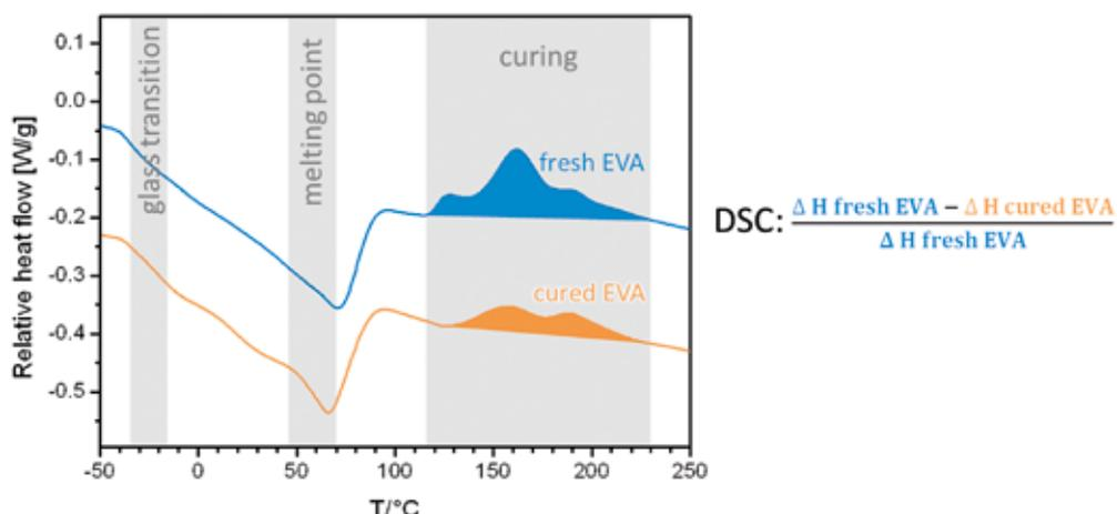
Figure 8. DSC measurement method [7].
