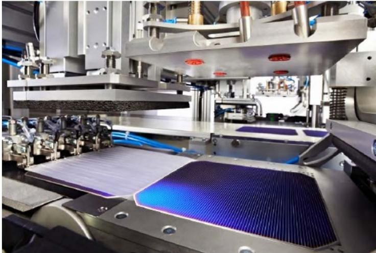
SWCT reduces silver consumption per heterojunction solar module by up to 75% and per PERC/PERT solar module by up to 65% which in turn reduces production costs for solar module manufacturers. Image: Meyer Burger
