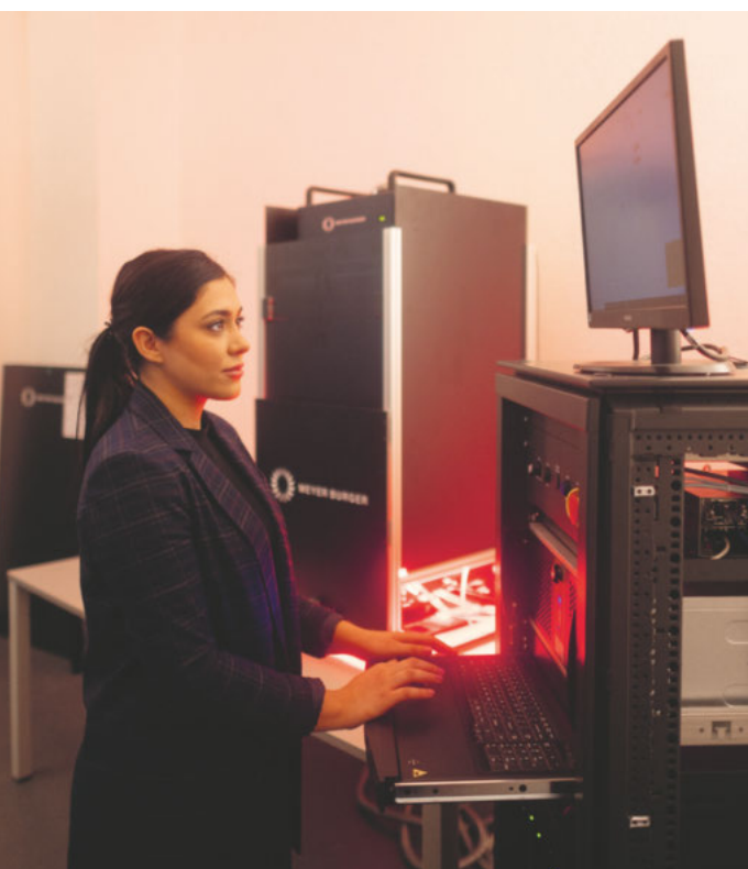
Neuchâtel Moment of truth: Pasan cell tester simulates sunlight and measures electrical power with maximum precision.
